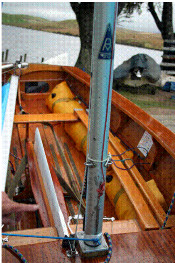
Figure 13: Deck mounted system with (white) control line led through Harken block and cam cleat. Red rope running line. Control pulley line and bungee attached to spreader bracket.
